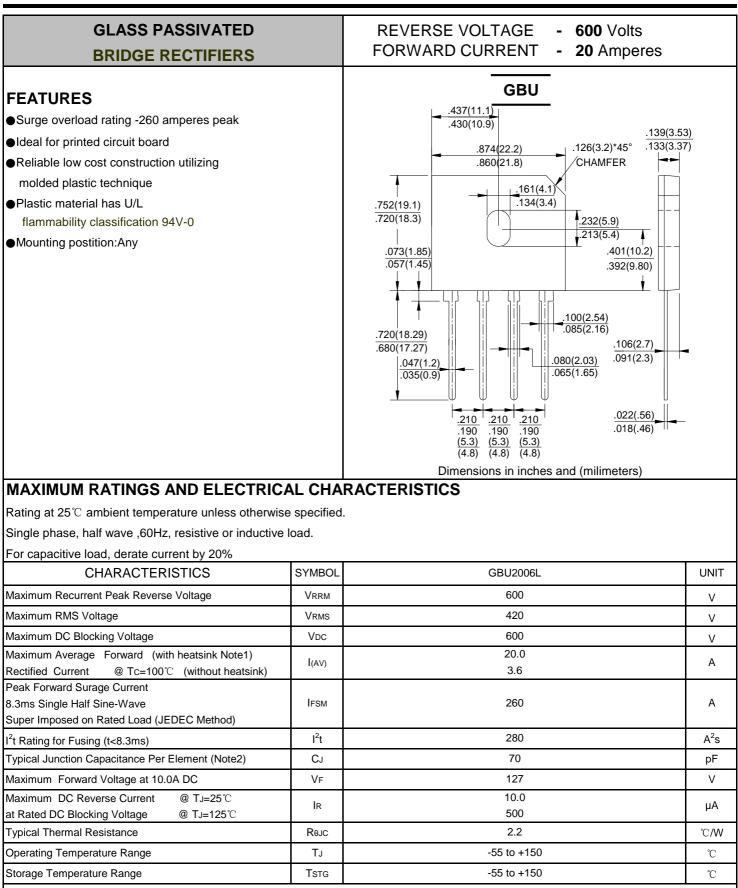
NOTES: 1.Device mounted on 100mm\*100mm\*1.6mm cu plate heatsink.
